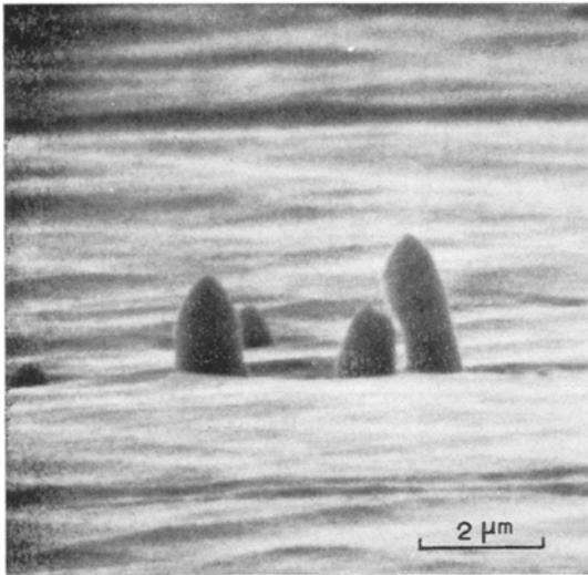
Figure 22 A micrograph showing the effect of ion etching a bent pillar structure. The side to the ion beam has started to develop into the characteristic slope while the pillar tip has become conical in shape, and asymmetric.
